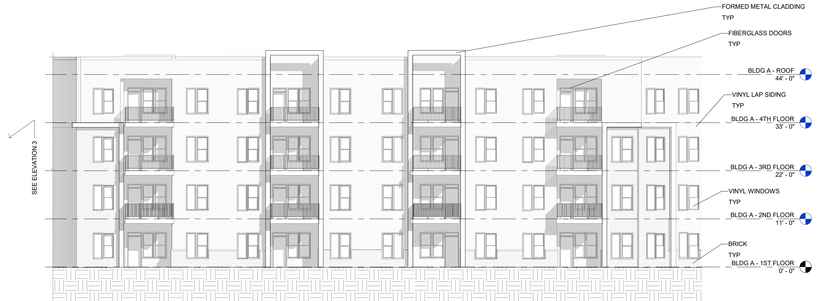
2 ELEVATION - BLDG A - SOUTH 3/32" = 1'-0"
