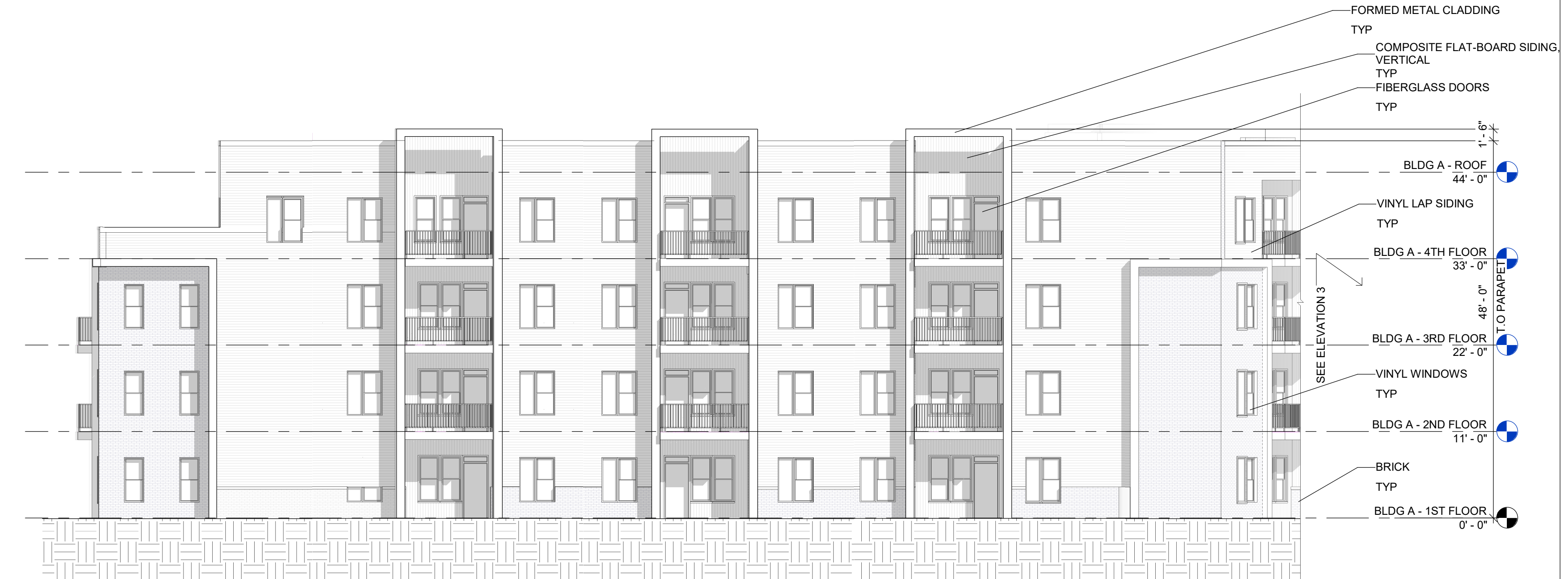
1 ELEVATION - BLDG A - SOUTHWEST 3/32" = 1'-0"
