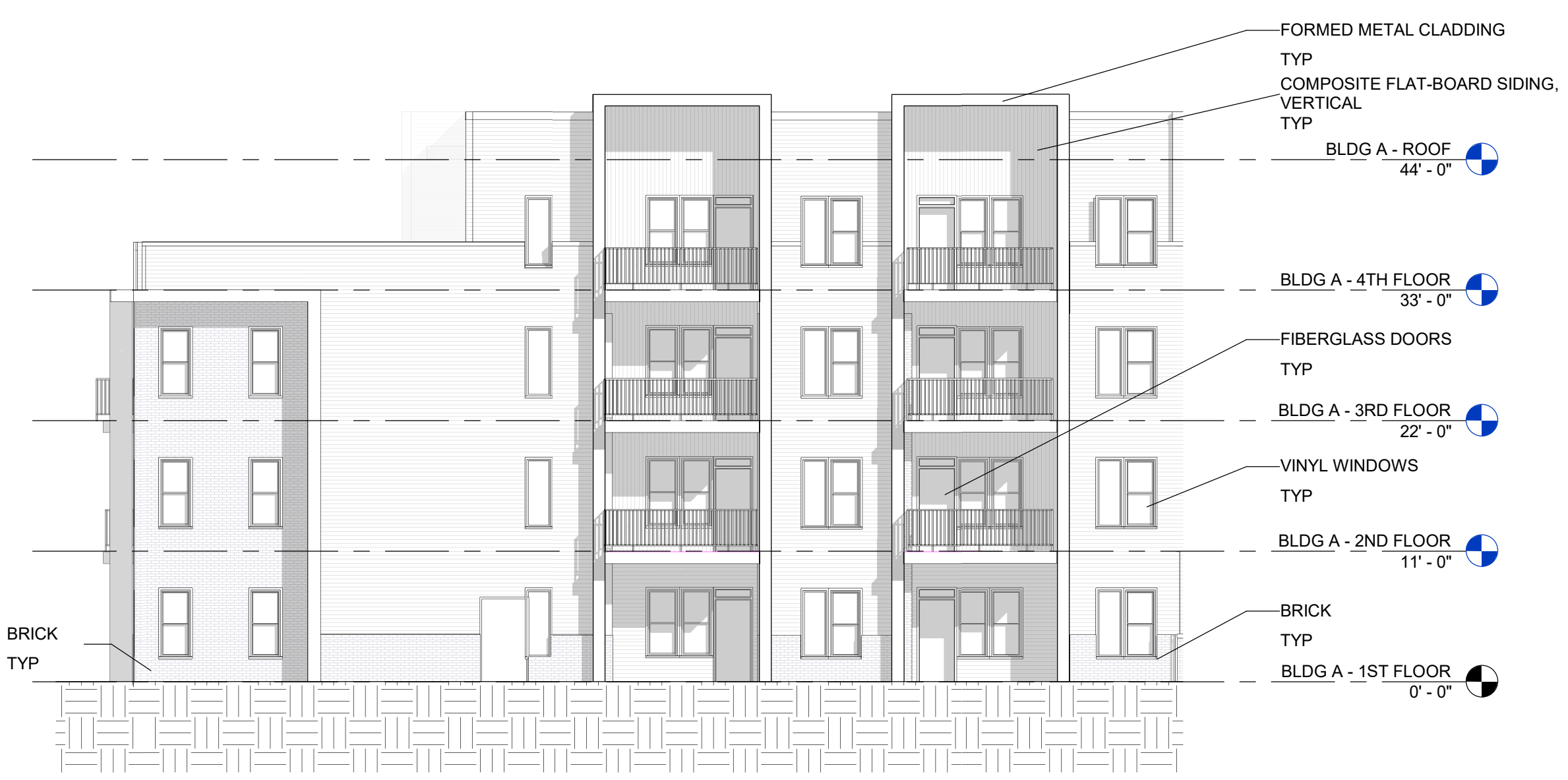
6 ELEVATION - BLDG A - NORTHEAST 3/32" = 1'-0"
