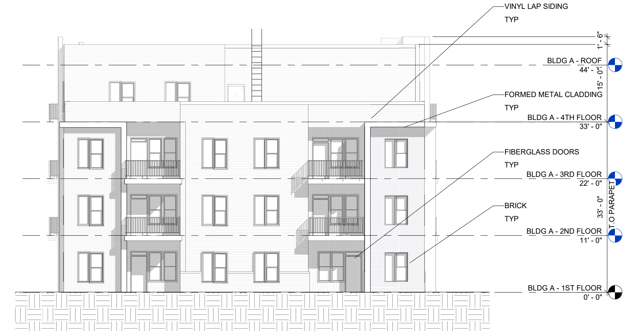
1 ELEVATION - BLDG A - EAST 3/32" = 1'-0"
