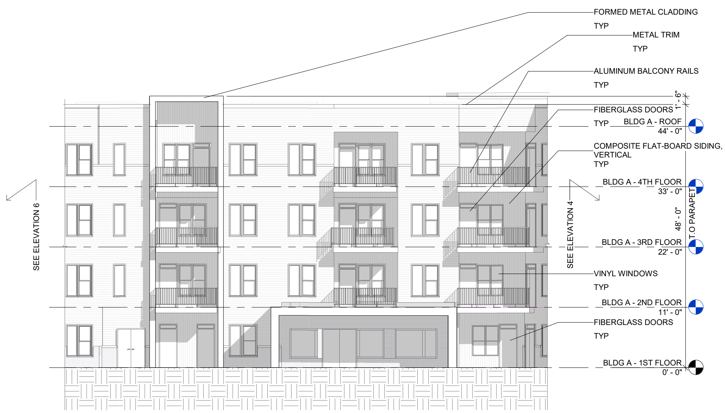
5 ELEVATION - BLDG A - NORTH 3/32" = 1'-0"
